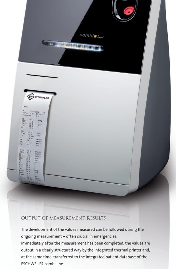
Additionally, the values measured can be transmitted directly to the central data management of the clinic or practice via an Ethernet connection (GDT or HL7).
